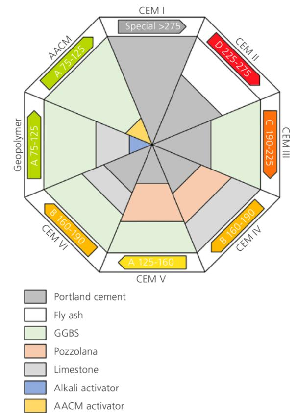
Fig 5.1: Typical carbon content of concretes made with different cements
