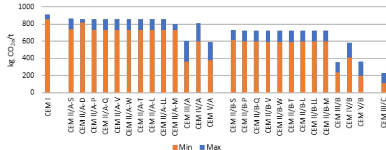
Fig 4.1: Cradle-to-gate carbon by cement types included in BS EN 197-1<sup>12</sup>
