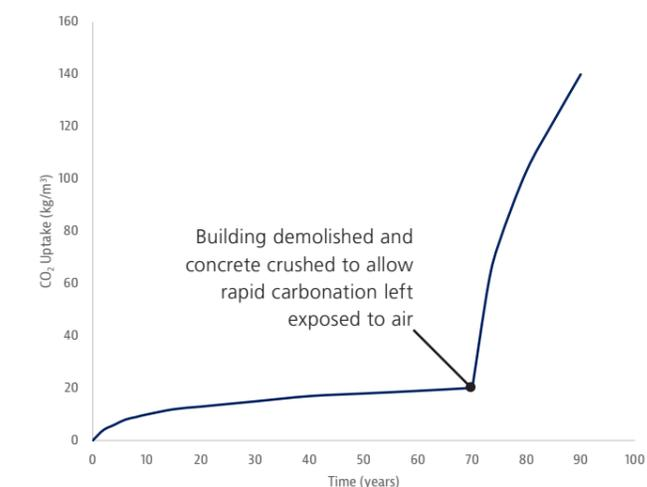
Fig 7.1: Indicative carbonation for typical concrete in a building, based on model estimating CO<sub>2</sub> uptake over time in CP III<sup>5</sup>
