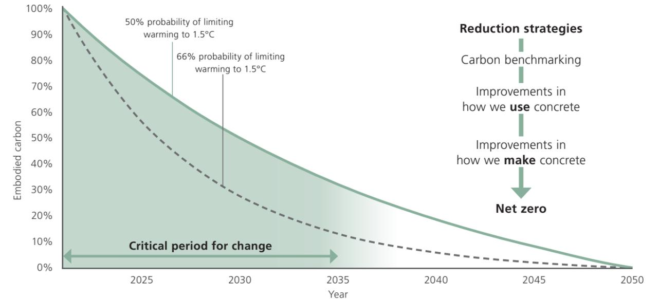
Fig 1: Idealised reduction rate for embodied carbon in concrete
