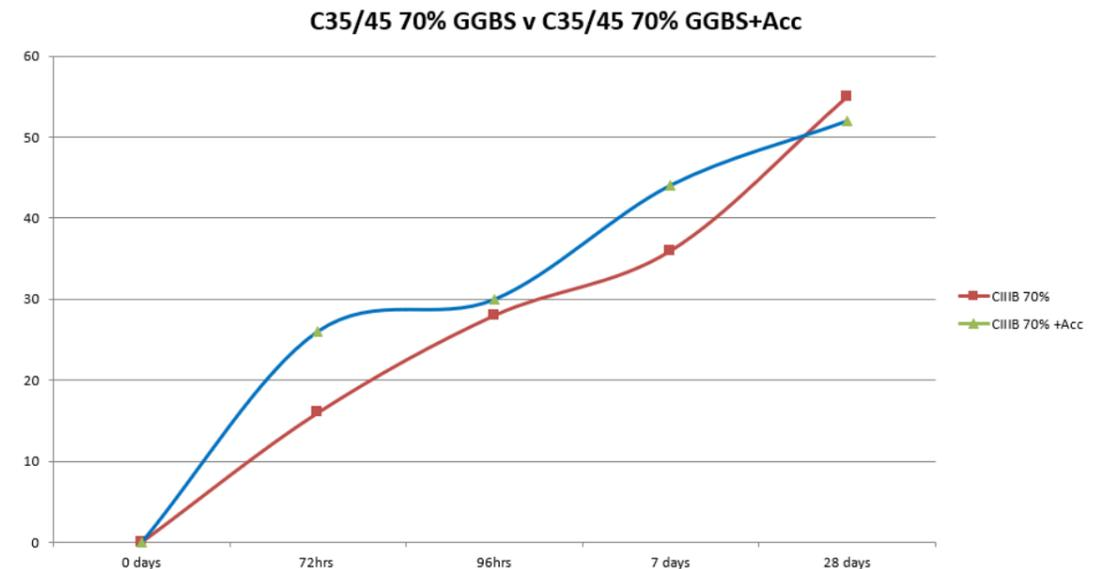
Fig 4.3: Impact of the use of accelerating additives to mitigate the use of SCMs
