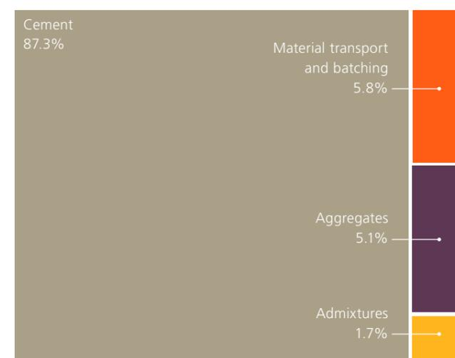
Fig 1.1: Distribution of embodied carbon in a typical structural concrete (RC25/30), LCA stages A1 to A3
