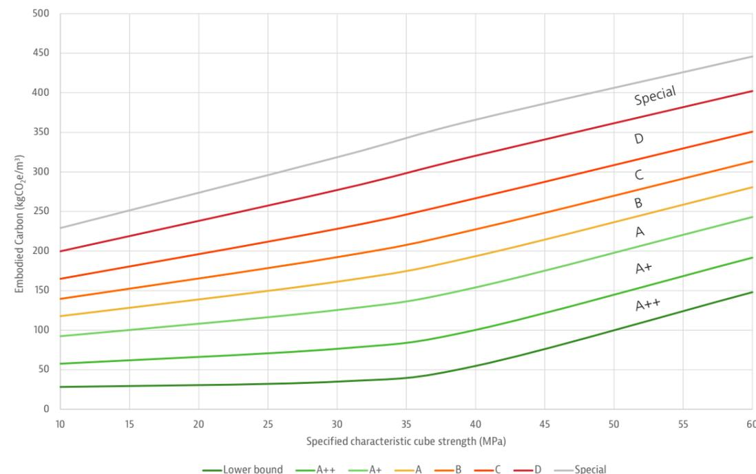
Fig 1.2: Ratings for embodied carbon, LCA stages A1 to A3
